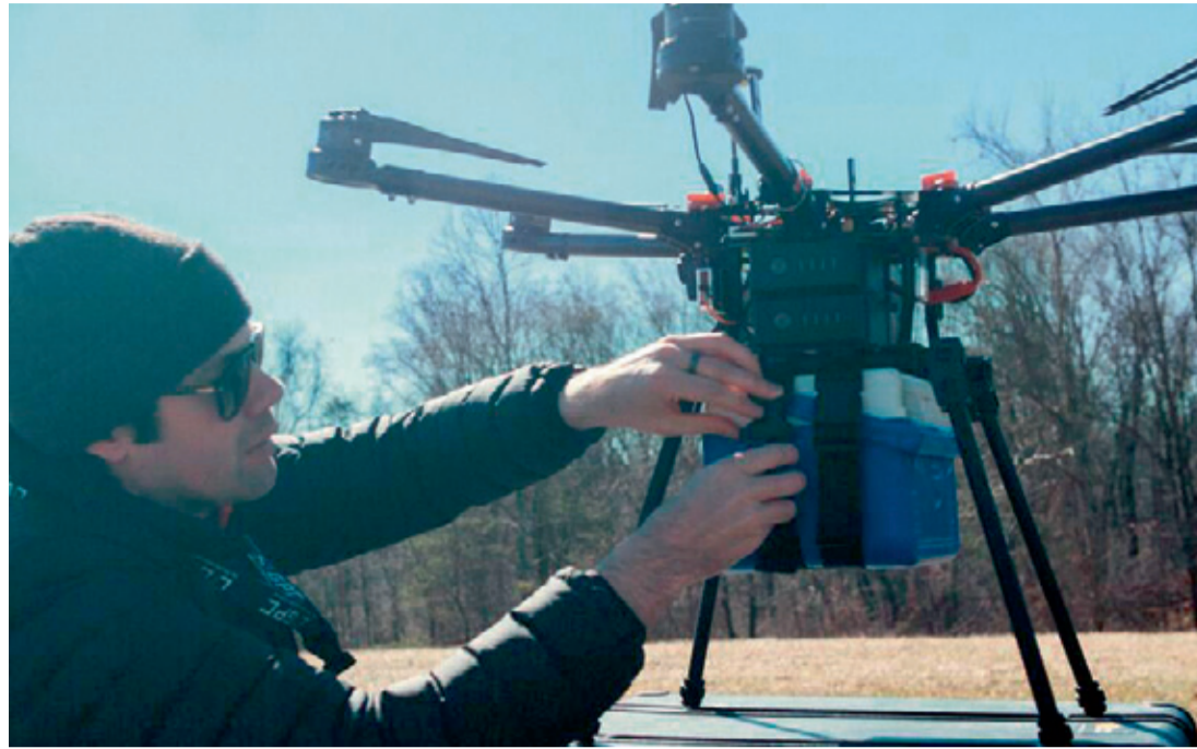
Blood products can maintain vital temperature and cellular integrity while being transported by specially-modified drones equipped with a hardened, temperature controlled cooler. — Supplied photo
